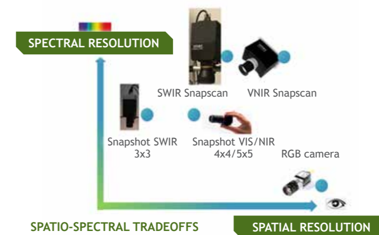
Figure 7/ Visualization of spatial-spectral trade-offs for camera systems
