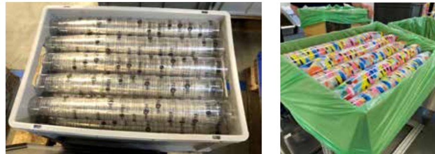
Figure 9/ Sleeve formation of cups for final storage
