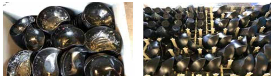
Figure 10/ Catering materials with special shapes gives difficulty when placed on the finger system.
