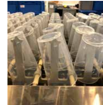
Figure 8/ Position of cups on finger-rest system
